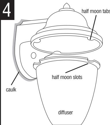
Attach diffuser by aligning half moon shaped cut out on diffuser with half moon tab on fixture and rotating diffuser counter clockwise until it is hand tight.
