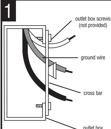
ATTACH cross bar to outlet box with outlet box screws (not provided).
