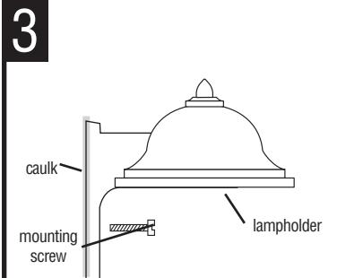
POSITION THE FIXTURE over the outlet box and secure in place with the mounting screw (provided).
