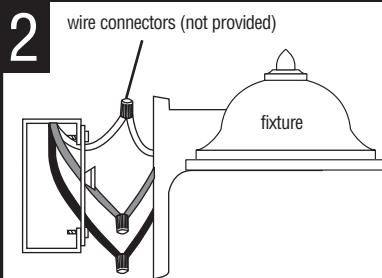
CONNECT THE WIRES. NOTE: Attach black fixture wire to black supply wire, white fixture wires to white supply wire. Do not mix them up. Use wire connectors (not provided). Connect green fixture ground wire(s) to ground wire from outlet box. NEVER CONNECT GROUND WIRE TO BLACK OR WHITE POWER SUPPLY WIRES.
