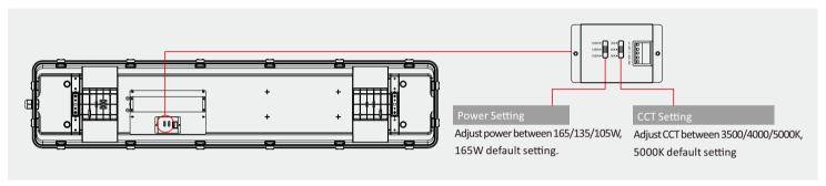
Note: Before Setting Power & CCT, release latches by pulling top of latch away from housing. Gently squeeze the buckle in and take out the PCB board (be careful not to touch the LEDs)
