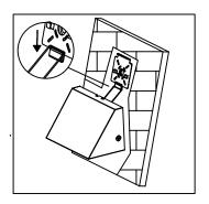
4) .After hanging the lamp on the mounting plate and tightening the screws, And put a waterproof glue seal between the bottom cover and the wall to prevent water from entering the lamp.
