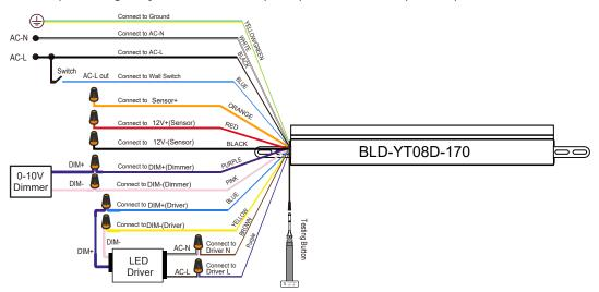
2. For luminaire with 0-10V LED driver, without using 0-10V dimmer (\* LED DRIVER INPUT POWER NOT GREATER THAN 60W). Emergency Inverter Dim+ (Blue), Driver Dim- (Yellow) has to connect with LED driver DIM+ and DIM-.
