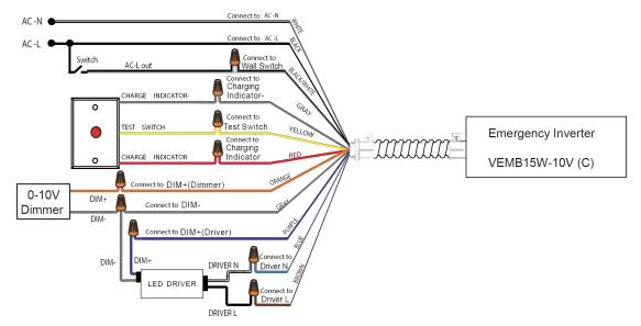
2. Emergency Solution with 0-10V LED driver, without using 0-10V dimmer (\* LED DRIVER INPUT POWER NOT GREATER THAN 80W)
