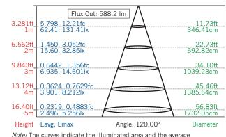
*Note:* The curves indicate the illuminated area and the average illumination when the luminaire is at a different distance.
