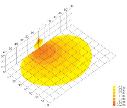
Ground mounted at 6" above ground, 10° above horizontal, shining towards building exterior wall at 20' away
