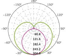
Maximum Candela = 1248.55 Located at Horizontal Angle = 0, Vertical Angle = 0
