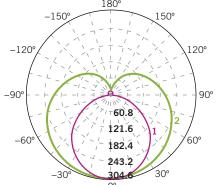
Maximum Candela = 1248.55 Located at Horizontal Angle = 0, Vertical Angle = 0
