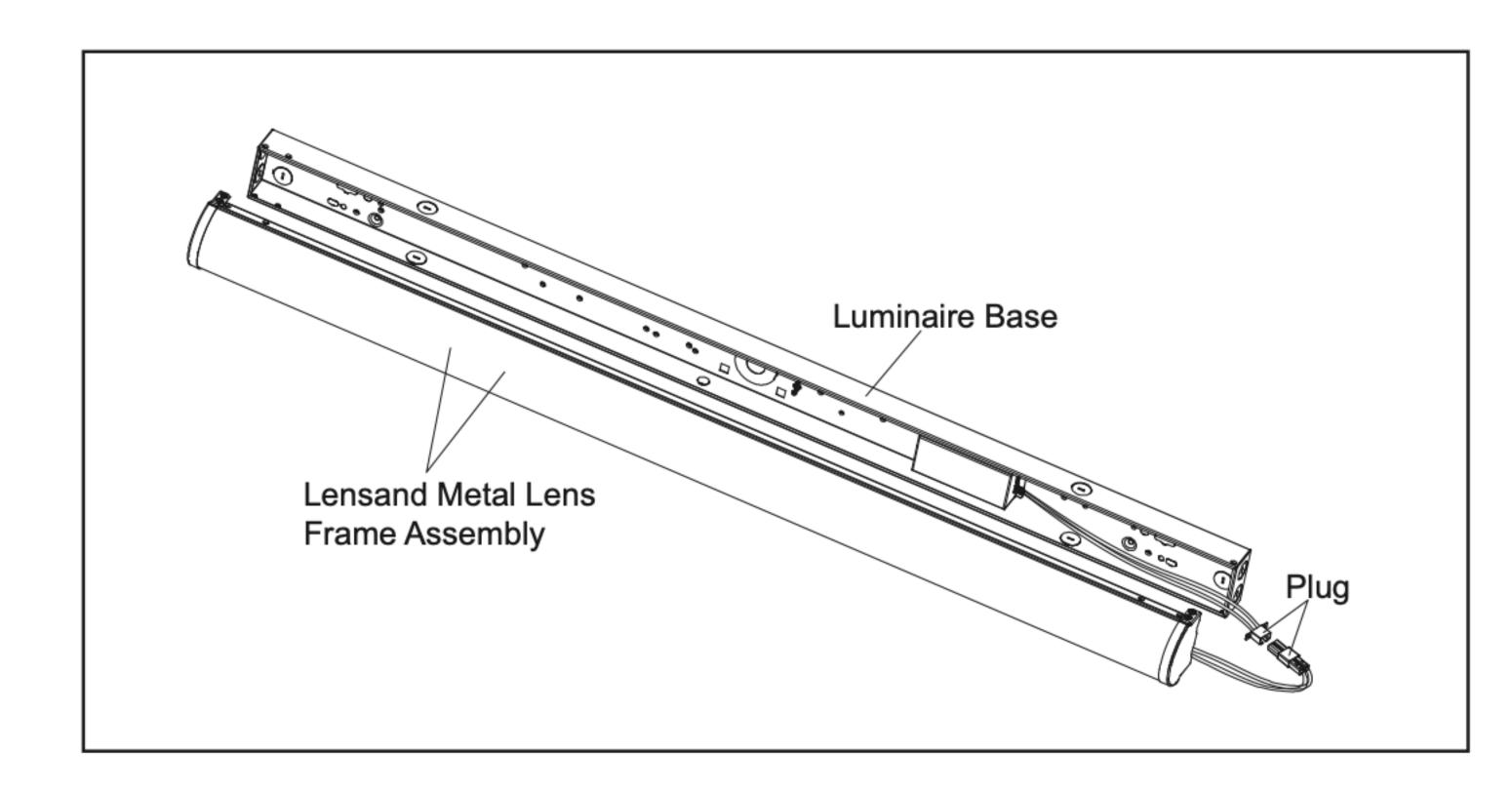
2. Disconnect the wire plug to start installation.
