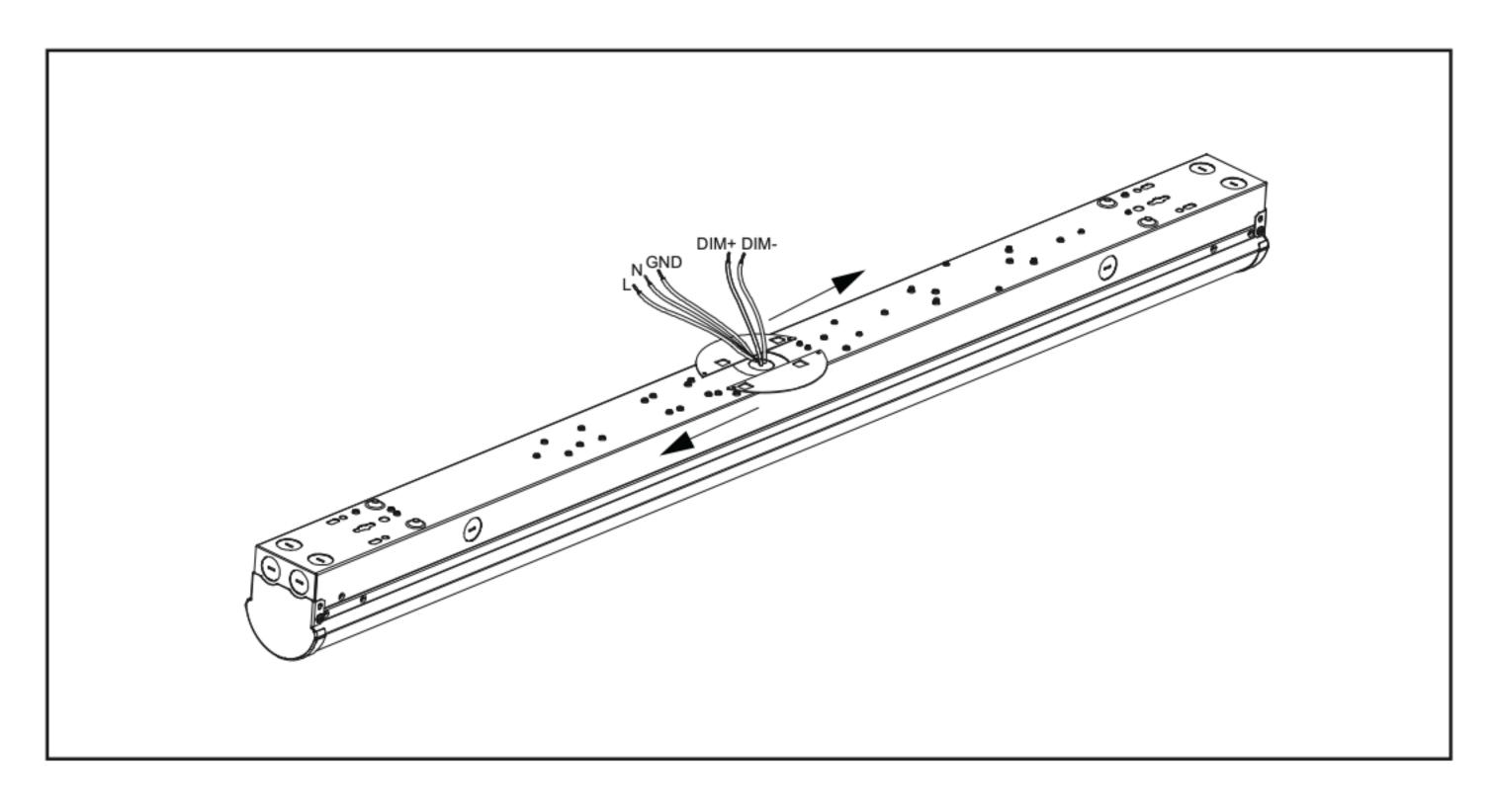
3. Install and lock the mounting plate on the luminaire base following the arrow.
