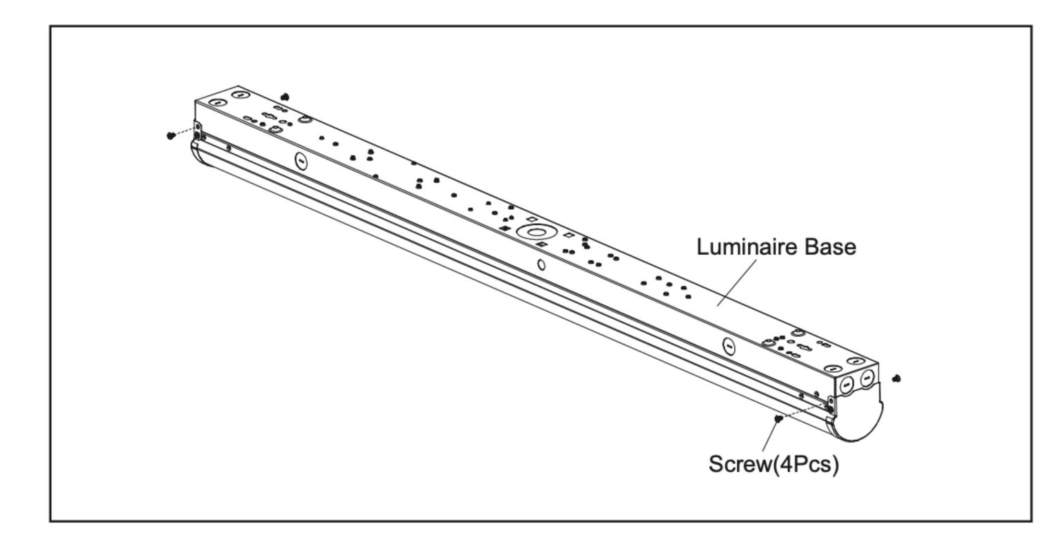
1. Unscrew the 4pcs screws on the back box of the luminaire or the luminaire base.
