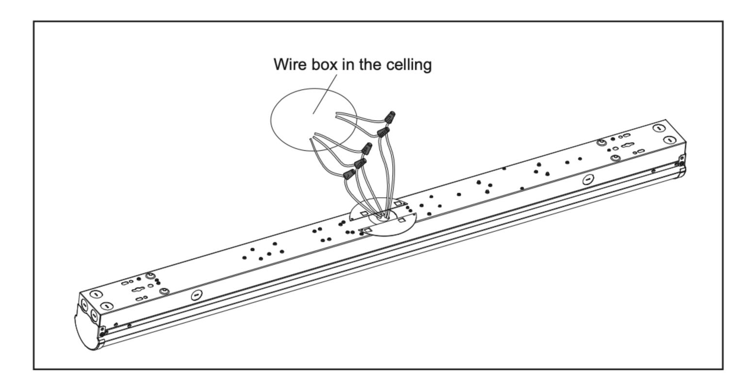
4. Connect the AC wires and dimming wires.
