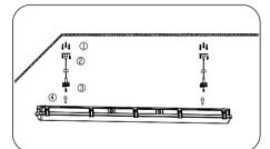
Secure suspended mounting kits to ceiling using 6-12 screws. Secure another side of suspended mounting kits to clips using 4-8 screws. Orient the luminaire so conduit fitting faces incoming supply power or conduit. Align the recesses and apply gentle upward pressure to secure luminaire onto both mounting clips.
