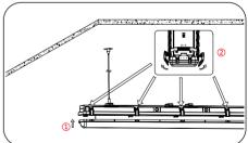
After align lens and bottom housing, turn off the luminaire. Secure lens to housing with lens latches.
