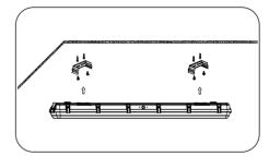
Secure mounting clips to ceiling using 4-8 screws. Space the clips 33.67 inches apart for 4 foot luminaire, or 37.8 inches apart for 8 foot luminaire. Orient the luminaire so conduit fitting faces incoming supply power or conduit. Align the recesses and apply gentle upward pressure to secure luminaire onto both mounting clips.
