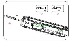
Separate the waterproof plug, and connect the input wire to the output wire of the power supply after passing through the plug and the outlet as shown in the figure.
