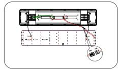
Disconnect the wire connecting the LED board and the driver to avoid unstable connection due to heavy suspension.
