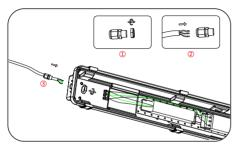
Separate the waterproof plug, and connect the input wire to the output wire of the power supply after passing through the plug and the outlet as shown in the figure.
