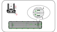
Release latches by pulling top of latch away from housing. Gently squeeze the buckle in and take out the PCB board (be careful not to touch the LEDs)..
