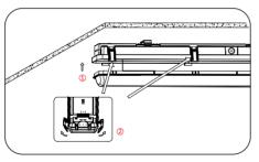
After align lens and bottom housing, turn off the luminaire. Secure lens to housing with lens latches.
