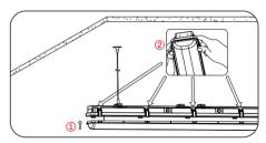
8. After align lens and bottom housing, turn off the luminaire. Secure lens to housing with lens
