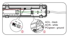
7. After the connection is completed, tighten the waterproof plug. Reconnect the wiring between the LED board and the driver
