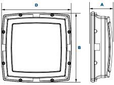
The LEPG Excel Square Bulkhead is designed to replace HID lighting systems up to 250w MH or HPS. The open door frame allows for maximum light output. Typical applications include office and public buildings, condominiums, schools, shopping malls, and hospitality. Recommended mounting heights are 8 to 20 feet.
