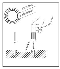
1) .According to the installation hole position on the lamp base, make 3 holes with diameter of 10MM on the ground and push the screw into the hole.
