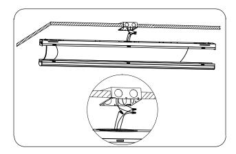
2.Fix the baffle on the lamp.
