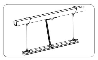
2.Attach V-hooks to the cable.
