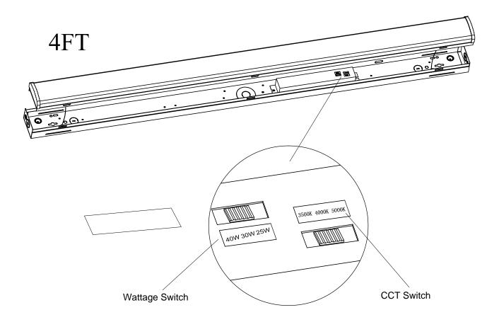
The end users may adjust the color temperature and lumen output respectively by the two DIP switch.Each DIP switch is accommodated with 3 options (left, middle and right ),corresponding to 3 color temperatures and 3 powers respectively, which can perform the desired color temperature and lumen output combination.
