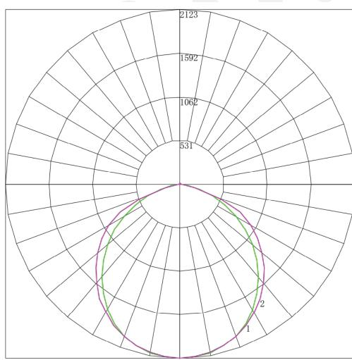
Maximum Candela =2123.31 Located at horizontal angle = 0, vertical angle = 0 #1 - Vertical Plane Through Horizontal Angles (0 - 180) # 2 - Vertical Plane Through Horizontal Angles (90 - 270)
