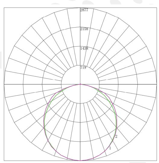
Maximum Candela =2876.733 Located At Horizontal Angle = 0, Vertical Angle = 0 # 1 - Vertical Plane Through Horizontal Angles (0 - 180) # 2 - Vertical Plane Through Horizontal Angles (90 - 270)
