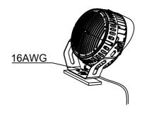
Connect the AC line, AC line for 16 AWG.
