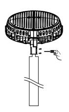
(1)Connect the AC line,AC line for 16 AWG.
