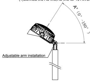
(2)Install the fixture on the pole.
