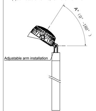
(2)Install the fixture on the pole.
