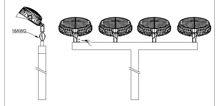
(1)Connect the AC line,AC line for 16 AWG.
