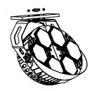
(1)Hold luminaire in place and install bolt, flat washers, and nut to securely fasten the fixture mounting bracket to the mounting structure.
