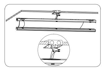
2.Fix the baffle on the lamp.
