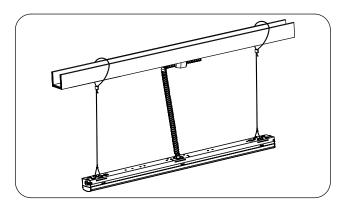
2.Attach V-hooks to the cable.
