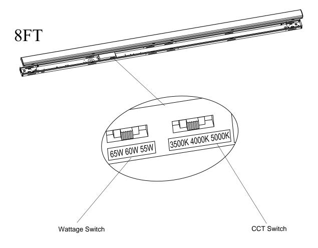
The end users may adjust the color temperature and lumen output respectively by the two DIP switch. Each DIP switch is accommodated with 3 options (left, middle and right), corresponding to 3 color temperatures and 3 powers respectively, which can perform the desired color temperature and lumen output combination.
